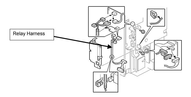
The relay harness is packed with some of the August and September production lots of the fax unit to fix a problem with the domestic version product. The harness is not mentioned in the service manual.
